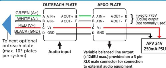
To connect Outreach plates to the balanced line level input of an amplifier that does not have an outreach socket, use an APV 24V 250mA regulated power supply and an APXO three pin XLR output plate with an appropriate lead. Outreach plates should be daisy-chained to the APXO and PSU using standard two pair audio cable (such as Belden 8723) as shown.
