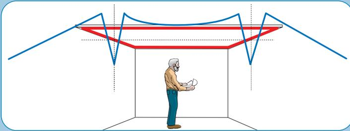
Logically, if we wanted to reduce the overspill we can move the loop into the room moving the overspill with it, thus:-
