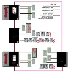
The Lexicomm ViLX-EX8 is a self contained enclosure housing a display, one to four dual line cards, an EN54-4:A2 2006 power supply & battery charger and is surface mounted, the small form factor makes it ideal for locating in electrical risers.
