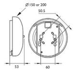
Mounting holes are provided to suit either BESA single gang installation boxes or for direct wall mounting
