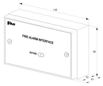
(All measurements shown are in millimeters)
