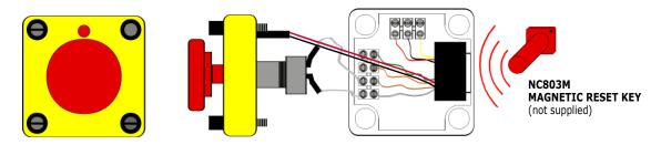
Designed for use with C-TEC's 800 Series Call System, the NC802DEWM is similar in appearance to an emergency stop type button. It's bright colour and water resistant qualities make it ideal for areas where the calling device must be easily identifiable by members of the public and for places where there are high levels of moisture (alongside swimming pools, jacuzzis, changing rooms, etc).
