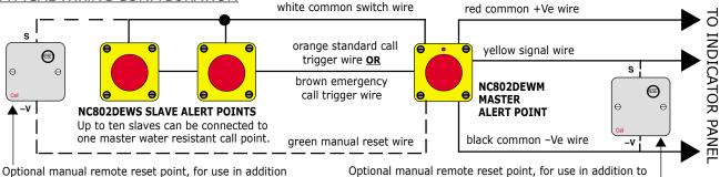
Optional manual remote reset point, for use in addition to (or instead of) the NC802DEWM's built-in magnetic reset facility. This reset point will reset standard <u>and</u> emergency calls. This device is not water resistant.
