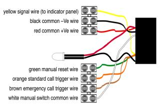
The remaining wires should be connected as shown in the Typical Wiring Configuration diagram below. Unused wires should always be terminated properly to ensure correct operation. Optional slave water resistant alert points (order code NC802DEWS) and remote reset points are also available for even greater flexibility. These should be connected to the NC802DEWM as shown below. Take care not to trap any wires when securing the alert point's front to it's back box.
