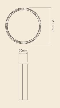
The Squashni presents the many qualities of the Roshni in the form of a base sounder for use with almost any available fire detector. The flat deck area can also be used with beacons to provide a compact audio-visual alarm device with the added economy of a single installation point.
